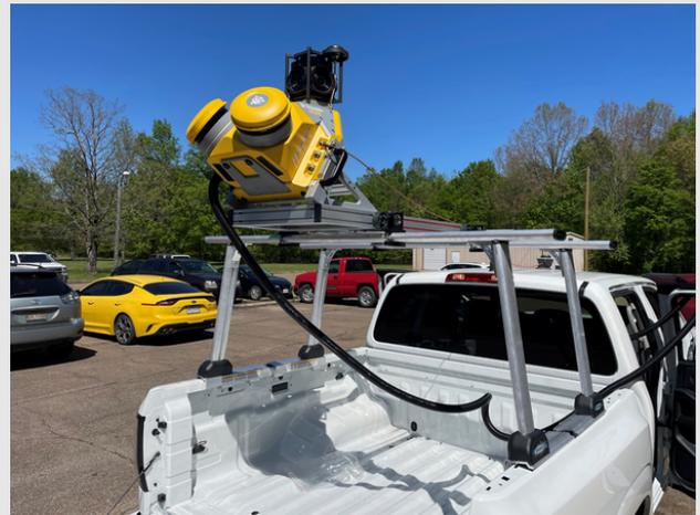
With these feature extractions, the new equipment can help the GTPDD counties with highway assets, utility assets, city assets, accurate ground models, engineering profiles and cross-sections, road surface information, addressing and more.
